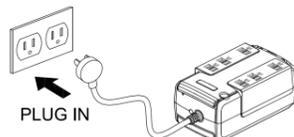
2. With the UPS unit turned off and unplugged, connect your equipment requiring battery backup into the battery power supplied outlets. Plug the other peripheral equipment (printer, scanner, speakers) into the full-time surge protection outlets. **DO NOT plug a laser printer, paper shredder, copier, space heater, vacuum, sump pump or other large electrical device into the "Battery and Surge Protected Outlets". The power demands of these devices will overload and possibly damage the unit.**
