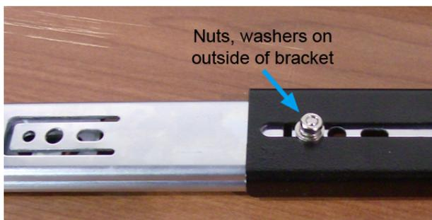
4. The rear rack mounting bracket can be fastened to the rails in the same manner as the front. These should not be fully tightened however, so they can be adjusted to the exact length needed to fit the rack/cabinet.
