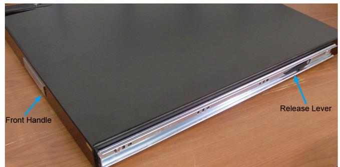
3. Attach the front rack mounting bracket to the sliding rail. The front bracket is the short bracket. Two screws will fasten the bracket to the rail. Make sure the screw is inserted from inside the rails, so the nuts and washers are on the outside.
