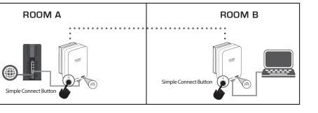
You can now connect another device using an Ethernet cable to the adapter. Verify that the Ethernet LED is lit. Your installation is completed.
