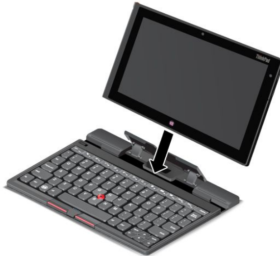
Figure 8. Installing the tablet into the Bluetooth keyboard
