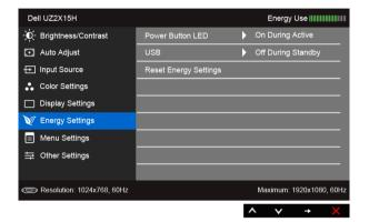
Power Button Allows you to set the power LED indicator On or Off to save energy. **LED** USB Allows you to enable or disable USB function during monitor
