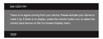
If either VGA, HDMI (MHL), or DP input is selected and the corresponding cable is not connected, a floating dialog box as shown below appears.
