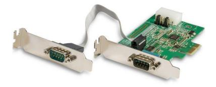
This RS232 Serial Adapter Card lets you add two RS232 (DB9) serial ports to your computer through a PCI Express (PCIe) slot. It enables you to interact with serial devices, such as card readers, printers, PIN pads, and modems, at speeds of up to 921.4Kbps.
