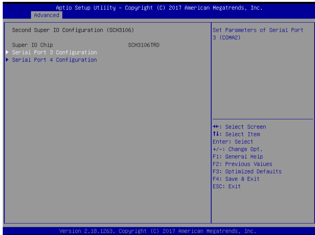
Figure 3.7 Second Serial Port Configuration(SCH3106)
