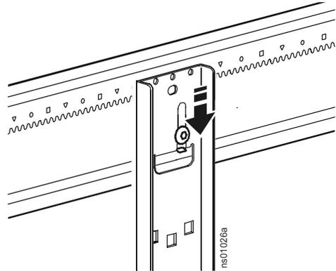
3. To align the vertical mounting flanges properly, note the symbol (for example, the diamond) visible through the hole on the top of the flange, and ensure that the same symbol is visible through the corresponding hole at the bottom of the flange. When the flanges are aligned properly, only one symbol is visible at a time through any of the holes.
