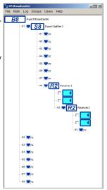
Indicates an available port on the DS128 transmitter. "NC" indicates a port with no Receiver unit connected to it.
