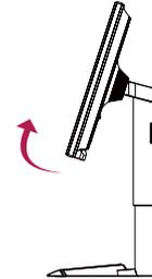
3 Rotate the monitor clockwise as shown in the figure.
