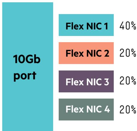
Virtual connections (also known as physical functions in NPAR) enable HPE ProLiant rack and tower servers with bandwidth management capabilities for each adapter. For example, a 10GbE port can be provisioned to operate as three separate physical functions: a full 8Gb FCoE stream and two separated 1GbE streams, such as management or VMotion. Dual-port 10GbE adapters deliver more flexibility to provision ports, reducing the need for multiple physical adapters performing the same functions.
