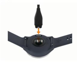
**3** Plug the USB cable into a power source to turn on the device (*Charging the Device*, page 9).
