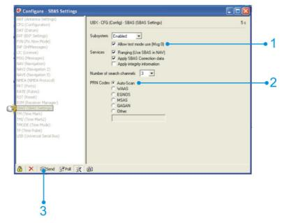
First, click on "SBAS" (Satellite Based Augmentation System). Then the SBAS settings item opens on the right. Click on the first free field before item 1 and 2. Then, click on item 3 "Sending". The changed data will then be transmitted to the receiver. Close the window. You will be asked if you want to save this setting. Click on YES.
