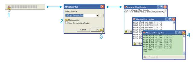
A small window with a small pull-down menu appears, in which you can see the validity of the data. Choose the desired validity period. Click on "Flash update", and then on OK. The UPDATE window opens and shows that the u-Center has loaded the data and is transmitting them to the NL-604P. When this process is finished, the window turns green, and the messages "SEND CANCEL" and "DONE" are displayed. This finishes the process.
