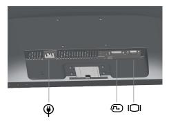
3. Connect one end of the analog signal cable to the monitor D-SUB connector and the other end to the computer.
