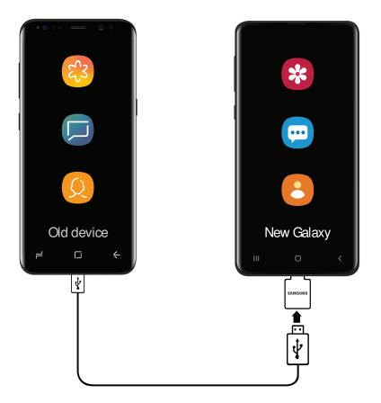
NOTE The USB option must be set to Media device (MTP) on the other device. Transferring content with a USB cable may increase battery consumption. Make sure your battery is fully charged.
