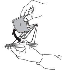
Fix the filter foam on the bottom filter. Clean the filter chamber of the dryer with a damp cloth or carefully with a vacuum cleaner. Insert the bottom filter again. Clap the filter handle down and close the bottom flap.
