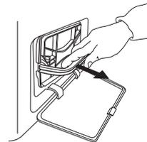
Remove the foam from the bottom filter, to clean it. Clean the filter foam and the filter by hand or under running water. Do not wash the filter foam in the washing machine. Wring out the filter foam. Do not insert it in the bottom filter dripping wet.
