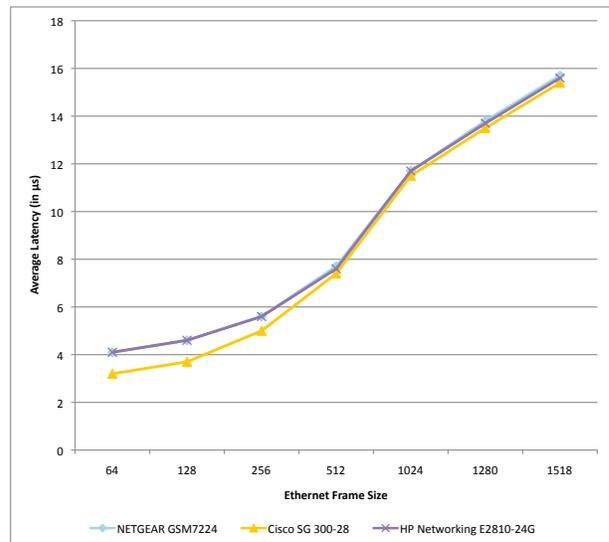
Note: Cisco's GbE switch has 28 ports where HP Networking and NETGEAR'S have 24 ports. For purposes of comparison, 24 ports were used on the Cisco switch. For the HP E2510-24 up to .5% of traffic was dropped at all frame sizes during the 100% load, latency test. For the D-Link DES-3528P approximately .5% of traffic was dropped at 64-byte frames only.
