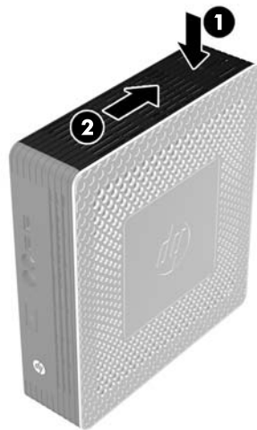
Figure 2-1 Removing the bottom cover
