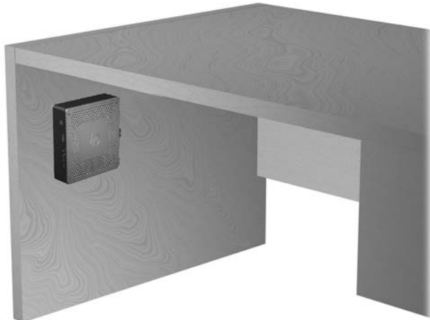
Figure C-7 Thin client mounted under desk
