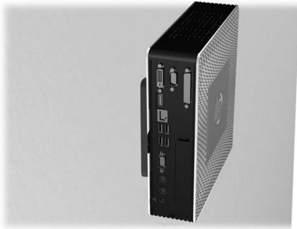
Figure C-6 Thin client mounted on wall
