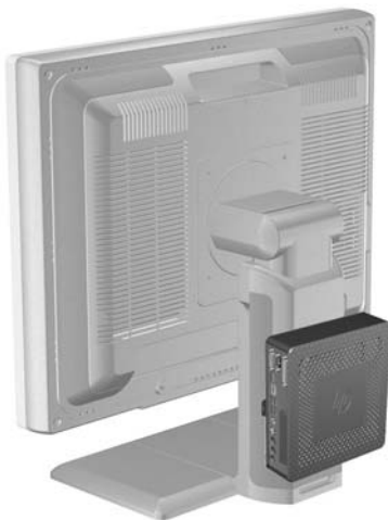
Figure C-5 Thin client mounted on back of monitor stand
