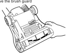
Remove brush assembly and check for wear on the belt. Loop the new belt around the motor and brush channel.
