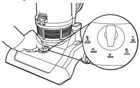
Ensure that the cleaner is in the upright (parked) position and move the selector to the required setting for the carpet type or floor covering.
