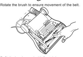
6 Refit the brush guard with 5 retaining screws.
