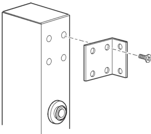
2. Attach the Rack PDU to a vertical mounting rail in the rear of the enclosure using two additional screws per bracket (not provided).
