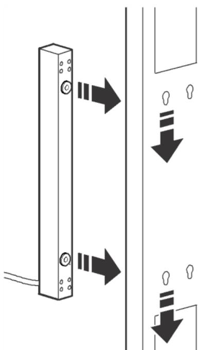
**NOTE:** You can mount two Rack PDUs on one side of the enclosure by using the toolless mounting method.
