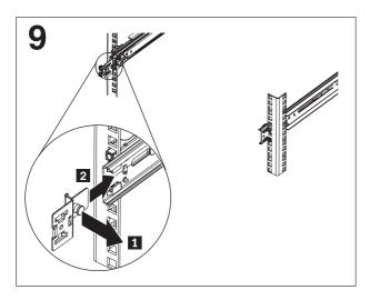
Pull out the mounting bracket pin 1 and slide the mounting bracket 2 into the slide rail onto which you are installing the cable-management arm. Push the bracket into the slide rail until the spring-loaded pin snaps into place.
