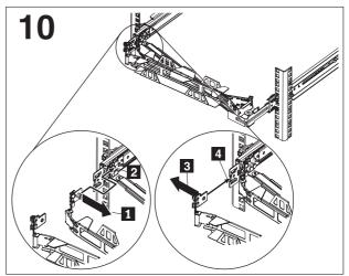
Place the cable-management arm on the support arm. Pull out the cable-management arm pin 1, and then slide the cable-management arm tab 2 into the slot on the inside of the slide rail. Push the tab until it snaps into place. Pull out the other cable-management arm pin 3, and then slide that cable management arm tab into the slot 4 on the outside of the slide rail. Push the tab until it snaps into place.
