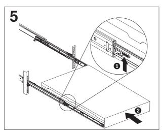
Lift the locking levers 1 on the slide rails and push the server 2 all the way into the rack until it either side of the server. This document shows it clicks into place.
