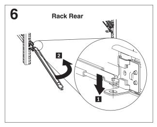
The cable-management arm can be installed on being installed on the left side. To install the cable-management arm on the right side, follow the instructions and install the hardware on the opposite side.
