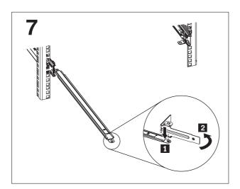
Install the L-shaped cable-management stop bracket To attach the other side of the support arm to the 1 on the unattached end of the support arm. Turn the bracket 2 to secure it to the support arm.
