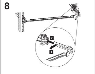
backside of the slide rail, pull the pin out **1**, and then slide the bracket 2 into the slide rail.
