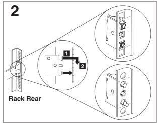
**Note:** When you install a 2U server, be sure to install the slide rails in the bottom U of the 2U area in the rack.
