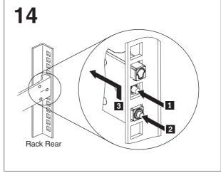
To remove the server from the rack, disconnect the cables from the rear of the server. Push the locking levers 1 forward, lift the front of the server up, and then pull the server out of the rack 3.
