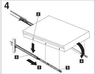
Pull the slide rails forward 1 until they click, two times, into place. Carefully lift the server and tilt it into position over the slide rails so that the rear nail heads 2 on the server line up with the rear slots 3 on the slide rails. Slide the server down until the rear nail heads slip into the two rear slots, and then slowly lower the front of the server 4 until the other nail heads slip into the other slots on the slide rails. Make sure that the front latch 5 slides over the nail heads.
