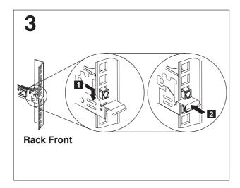
Pull the slide rail forward and insert the two pins on the front of the rail into the two lower holes in the U on the front of the rack. Drop the rail into place until it clicks. Push the front latch in all the way.
