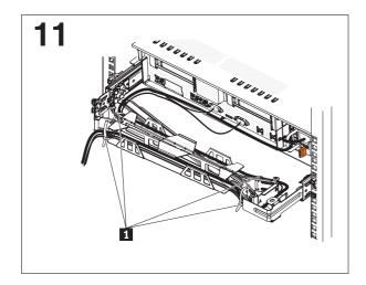
Attach the power cords and other cables to the rear of the server (including keyboard, monitor, and mouse cables, if required). Route the cables and power cords on the cable-management arm 1 and secure them with cable ties or hook-and-loop fasteners.
