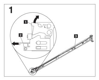
Each slide rail is marked with either an R (right) or an L (left). Select one of the slide rails and push up on the front moveable tab 1; then, pull out the front latch 2 to slide out the front side rail. If a thumbscrew is installed in the slide rail 3, remove it.
