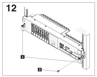
Slide the server into the rack until it snaps into place. To slide the server out of the rack, press on the release latches 1.
