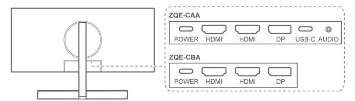
Open the protective cover on the bottom part of the monitor rear to view the ports. You can connect the monitor to a device such as a computer based on the cable type.
