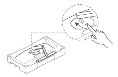
A Before installing the base support, ensure that there are no objects made of iron attached to the support at the rear of the monitor, otherwise a short circuit may occur.
