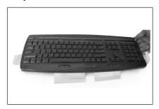
Gently lay cover over keyboard and align cover with the keys.
