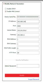
Figure 3-5 Modify the IP Address
