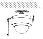
Figure 2-3 Secure the Camera to the Adapter Plate
