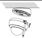
Figure 2-7 Secure the Camera to the Adapter Plate
