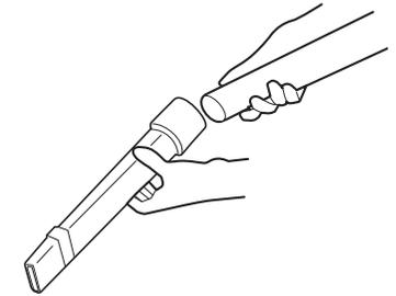
Check the hose by removing it from the cleaner, stretching it to full length.
