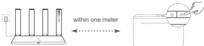
Step 2: When the indicator on the HUAWEI CPE starts to flash, press the H button on it. Wait until the indicator on the router shows that the router is connected to the network.
