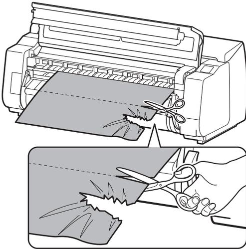
Pull the jammed portion out toward the front. Use scissors or a cutting tool to cut away the printed or wrinkled portion.
