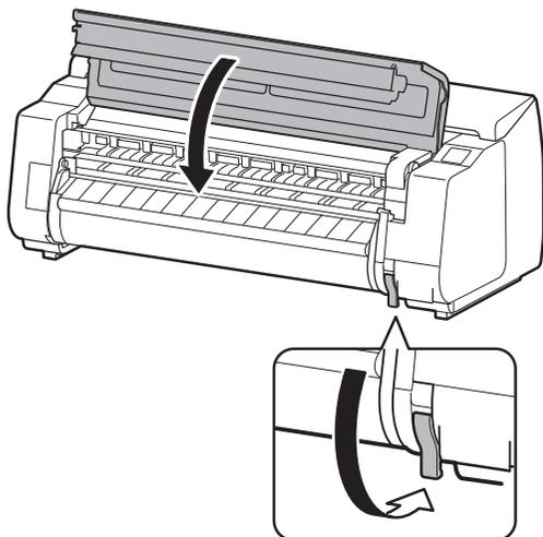
Lower the release lever and close the top cover.
