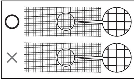
Once the print head cleaning has finished, print and check the nozzle check pattern.
