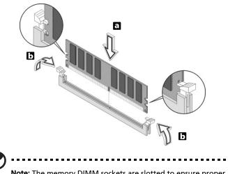
**Note:** The memory DIMM sockets are slotted to ensure proper installation. If you insert a memory DIMM but it does not fit easily into the socket, turn the memory DIMM around and try to insert it again.
