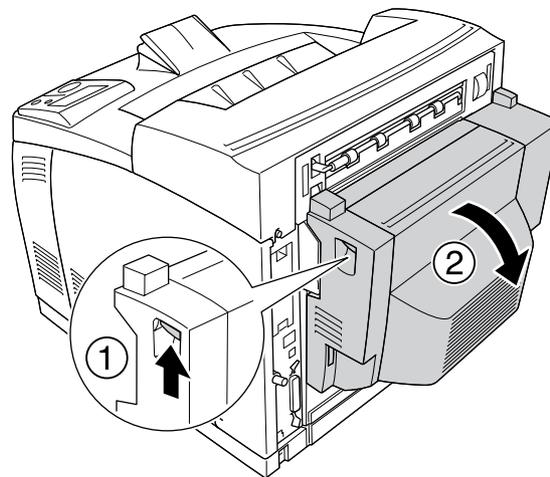
4. Attach the duplex unit connector cover and the upper option cover to cover B.
