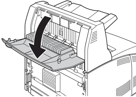
2. Remove any paper you find jammed inside the Stacker as shown in the illustration below.
