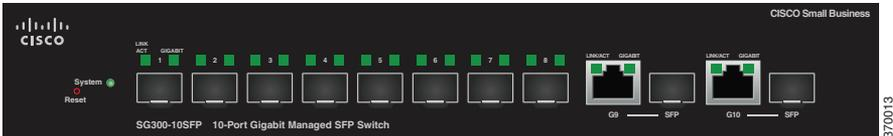
**RJ-45 Ethernet Ports**—Use these ports to connect network devices, such as computers, printers, and access points, to the switch.
