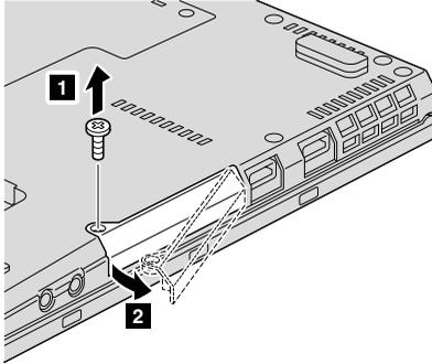
5. Remove the drive by pulling out the tab (an SSD is shown in figure).
