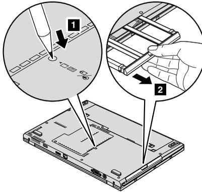
4. To put the travel cover in place, insert it into the slot until you hear the click of the release button.
