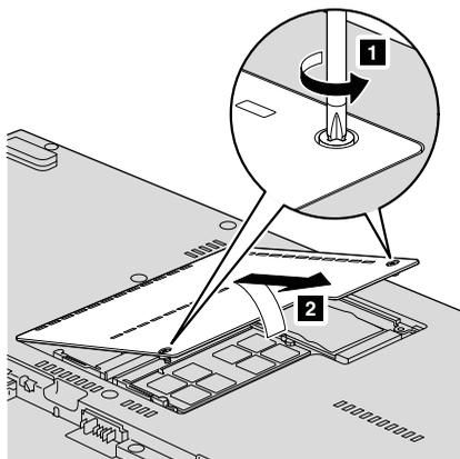
6. If two SO-DIMMs are already installed in the memory slot, remove one of them to make room for the new one by pressing out on the latches **1** on both edges of the socket at the same time, and pulling out the SO-DIMM **2**. Be sure to save the old SO-DIMM for future use.
