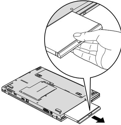
4. Insert the second battery in the slot, and then press it firmly.
