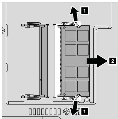
7. With the notched end of the SO-DIMM toward the contact edge side of the socket, firmly insert the SO-DIMM into the socket at an angle of about 20 degrees **1**; then pivot it downward until it snaps into place **2**.
