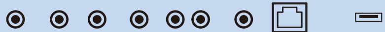
RS232 IN RS232 OUT IR-IN IR-OUT AUDIO OUT PC LINE IN RJ45 USB 2.0 5V/0.5A
