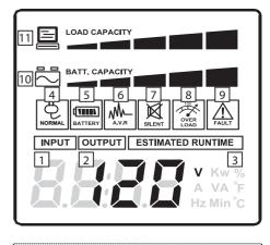
The LCD displays detailed information on the UPS status and current power conditions to alert you to potential power problems before the affect your equipment. Note! All related UPS information is based on that you should turn on the UPS.
