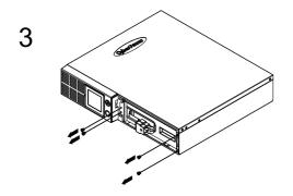
Remove the four retaining screws.
