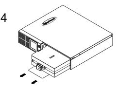
Insert the new battery pack. Assemble the screws, cable and front panel in the reverse sequence of above steps.\* Recharge the unit for 18 hours to ensure the UPS performs expected runtime.
