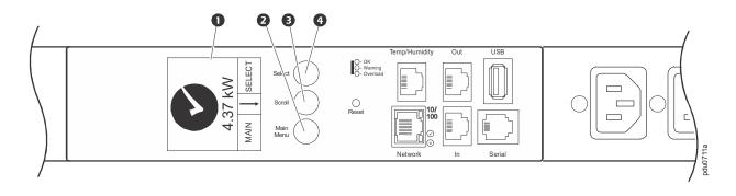
**NOTE:** Your Rack PDU is configured so the display backlight turns off after 10 minutes of inactivity. The backlight can be turned on by depressing any button below the display.
