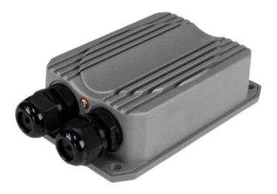
Take wireless connectivity to the great outdoors - through rain, snow or other extreme conditions - with this IP67-certified wireless access point. Tough and dependable, the 5GHz wireless AP lets you create or extend your wireless coverage, using an existing wired or wireless network, to connect across large open spaces and maximize throughput in your Wi-Fi network.
