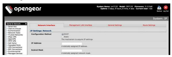
The second network port (*NET2*) is inactive by default. It can be set up for failover/OoB access (refer to the *User Manual*) or as a management LAN gateway. To activate:
