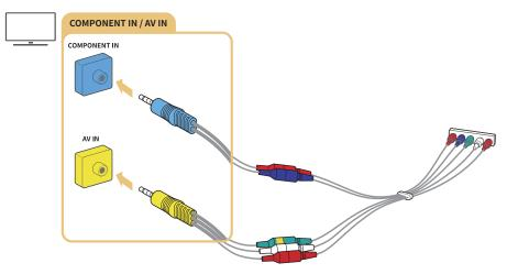
To use component equipment, connect both a component cable(blue) and an AV cable (yellow).
