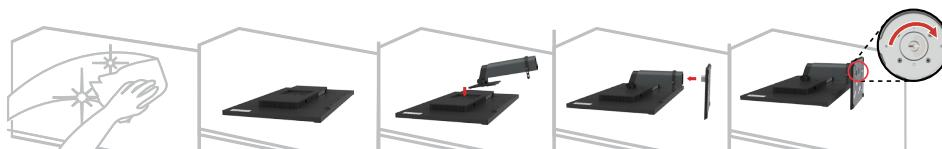
1. Carefully lay the monitor on a flat surface.
