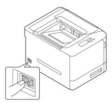
This displays the screen showing that the machine is running the start-up process. When **Message Window** appears in the [READY], it indicates that this machine is ready to run.
