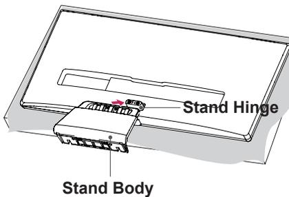
4 Tighten two screws into the back of the stand body .
