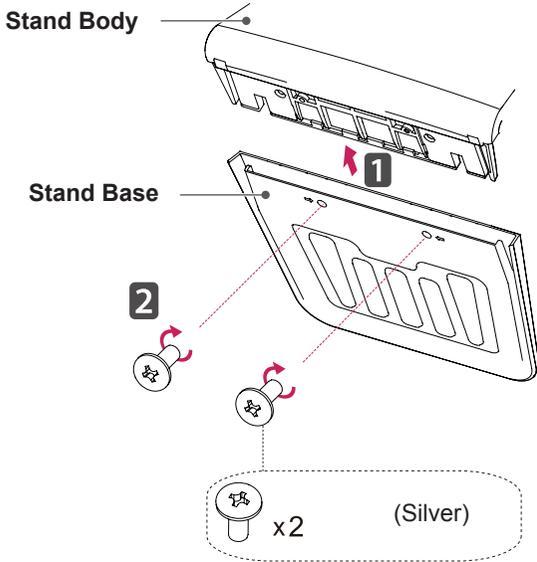
3 Check the direction of the stand body (front, back) and then mount the stand body onto the stand hinge.
