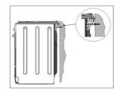
! In order to prevent accidental tipping of the appliance, for example by a child climbing onto the oven door, the supplied safety chain MUST be installed!
