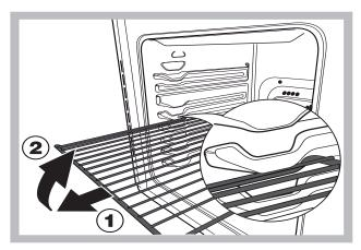
To reposition the telescopic runners unclip the runners from position, move them to the position you require and re-clip them to secure.
