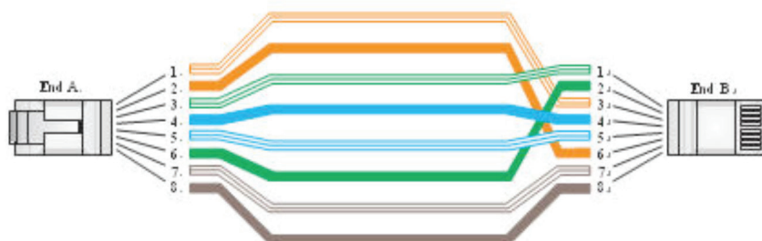
Figure 9-3. EIA/TIA 568B RJ-45 Wiring Standard 10/100BASE-TX Crossover Cable.
