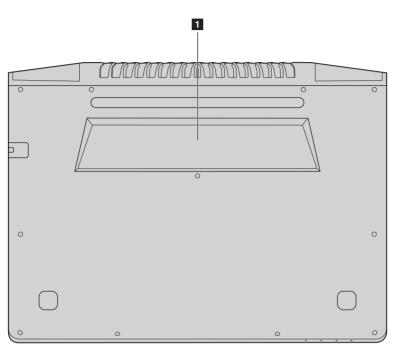
**Ventilation slots** Allow air to enter the computer for cooling.
