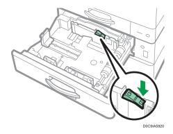
4. While pressing down the release lever of the side fence, slide the side fences outward.
