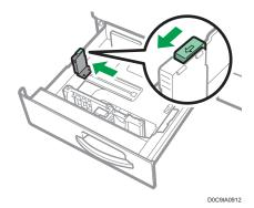
Rotate the fixing screw of the stopper 90 degrees counterclockwise with a coin or similar object and remove the stopper.
