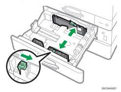
5. While pinching the release lever of the end fence, slide the end fence outward.
