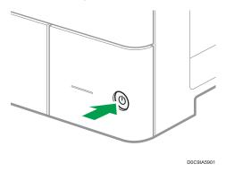
The main power indicator on the right side of the control panel turns off. The main power turns off automatically after the machine has shut down properly.
