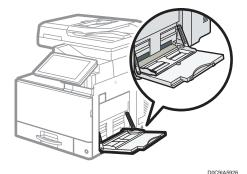
When loading paper larger than A4 or  $8^{1}/_{2} \times 11$  size, pull out the extender.
