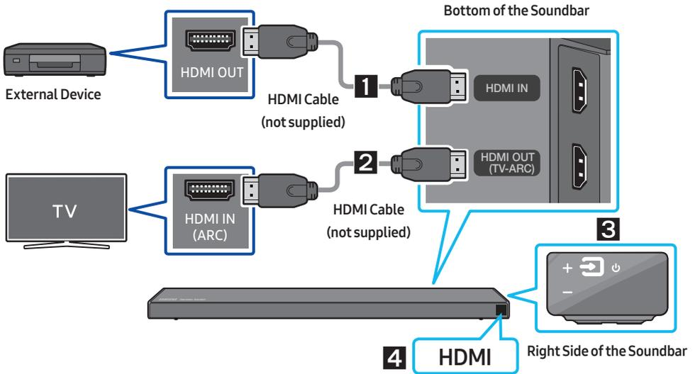
1. Connect an HDMI cable (not supplied) from the **HDMI IN** jack on the back of the product to the HDMI OUT jack on your digital device.
