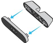
2. Use the 2 supplied **Screws** to fix the two **Holder-Feet** to the Wall Mount assembly on the bottom panel of the Soundbar.
