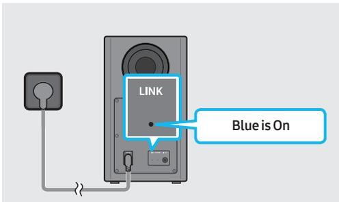
The LINK LED indicator stops blinking and glows a solid blue when a connection is established between the Soundbar and the Wireless Subwoofer.
