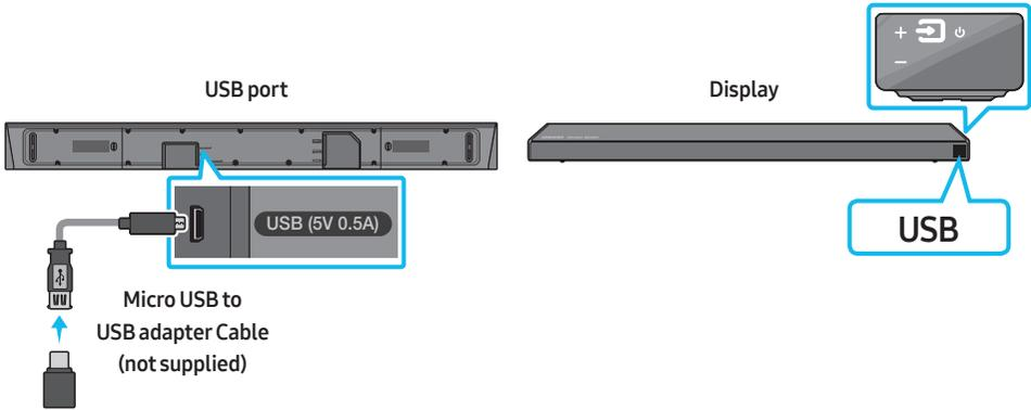
1. Connect a Micro USB to USB adapter cable with a male USB 2.0 Micro USB plug (Type B) on one end and a standard female 2.0 USB jack (Type A) on the other end to the micro USB jack on your Soundbar.
