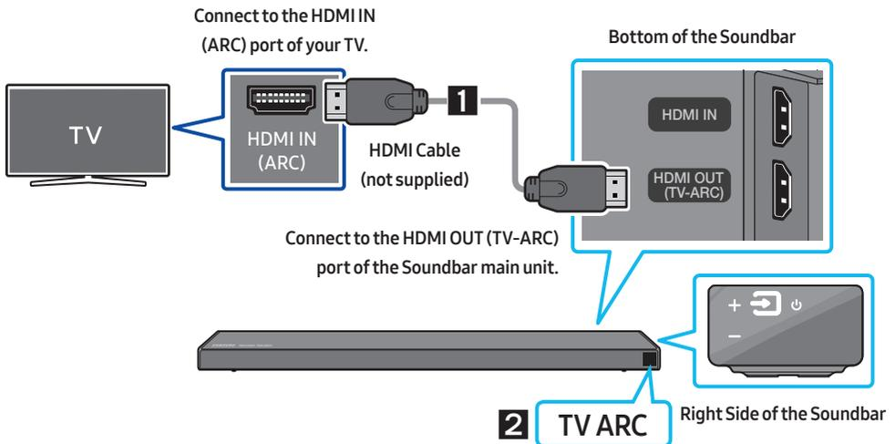
1. With the Soundbar and TV turned on, connect the HDMI cable (not supplied) as shown in the figure.
