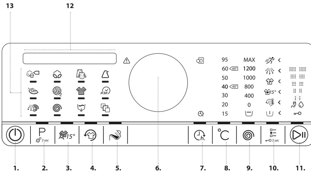
1. On/Off button (Reset/Drain if pressed and held down)
