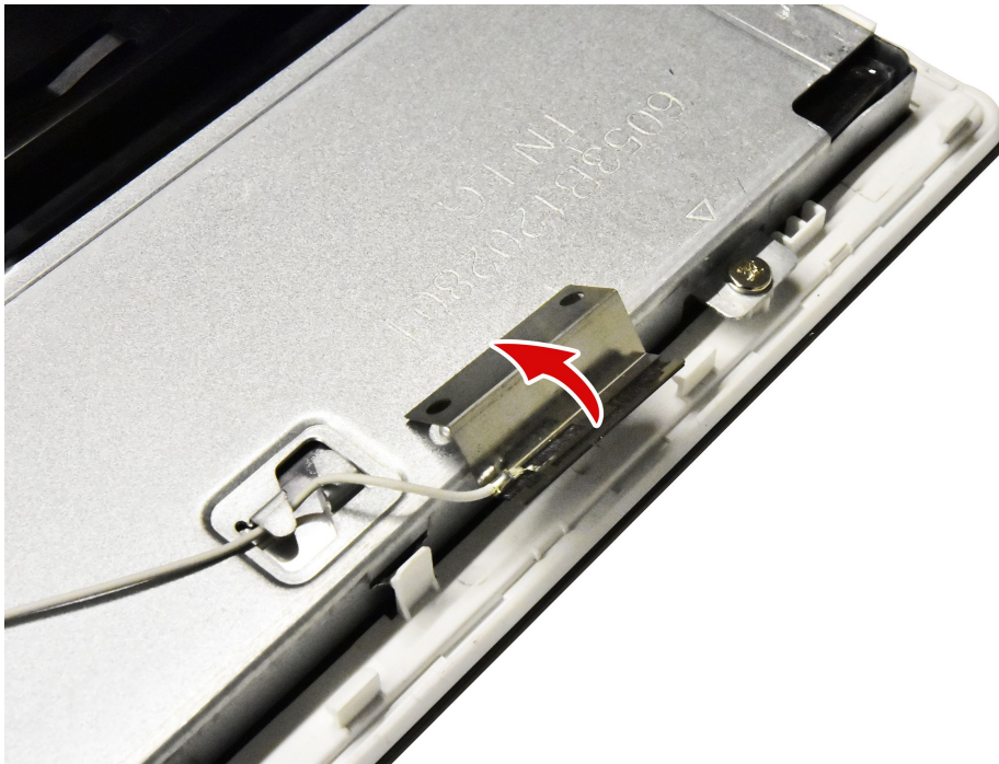
Step 23. Remove the touch control cable as shown.
