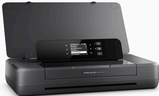
The TROY 200 Mobile MICR Printer is an ideal solution for businesses who need a mobile check printing solution. The portability of this unit is its most unique quality, providing satellite, mobile, and remote office locations with the ability to print checks on the go. The 200 Mobile features print speeds up to 20 pages per minute and a 50 sheet input tray.
