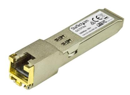
This StarTech.com Gigabit Copper SFP is a TAA compliant transceiver module, equivalent to the Cisco GLC-T. Built to exacting specifications and fully tested to ensure maximum performance, this high-quality SFP transceiver module can be installed into Cisco® switches and routers that support the GLC-T SFP transceiver module, as well as other major brands of networking equipment.
