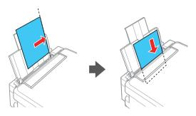
**3** Slide the edge guide against the paper, but not too tightly, and flip the feeder guard back.
