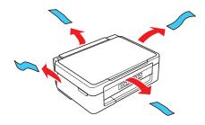
**2** Lift up the scanner unit and remove all protective materials from inside the product.
